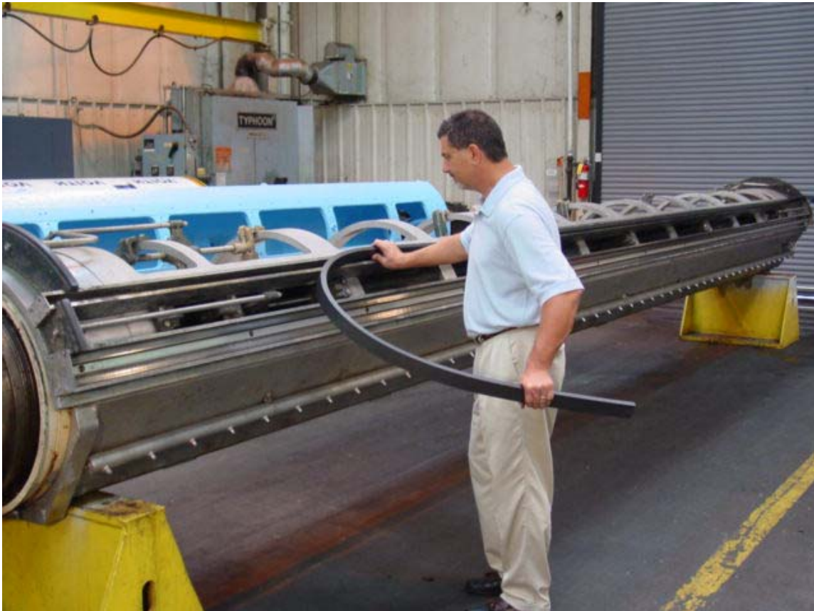
New flexible rubber graphite being installed
