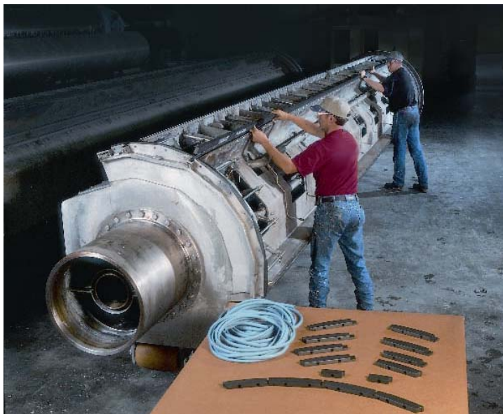
Large multi-zone suction box with classic RG seals, deckles and tubes.
