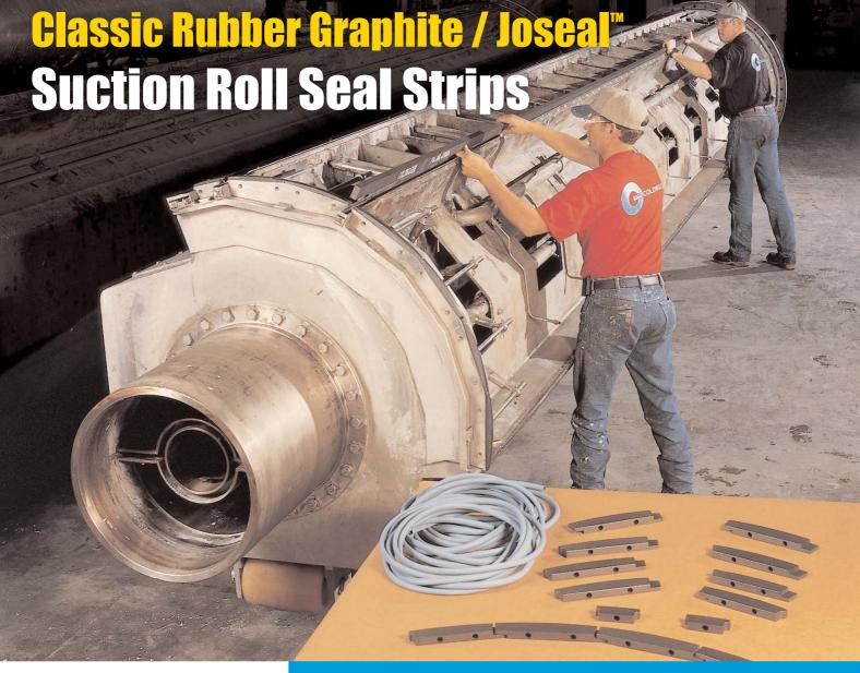
Our technicians can custom fit the seals to the roll. Custom fit seals can greatly improve running intervals (2 years or more) and significantly reduce horsepower consumption (up to 100 amps less per roll).
